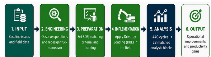
Figure 1. Field-based Drive-by Loading evaluation framework
