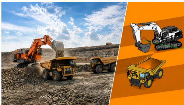
Figure 3. Existing single side loading configuration
