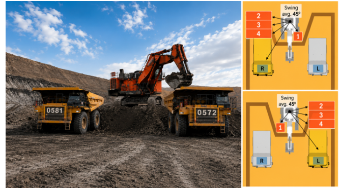
Figure 4. Double Side Loading Configuration Implemented at the Study Site
