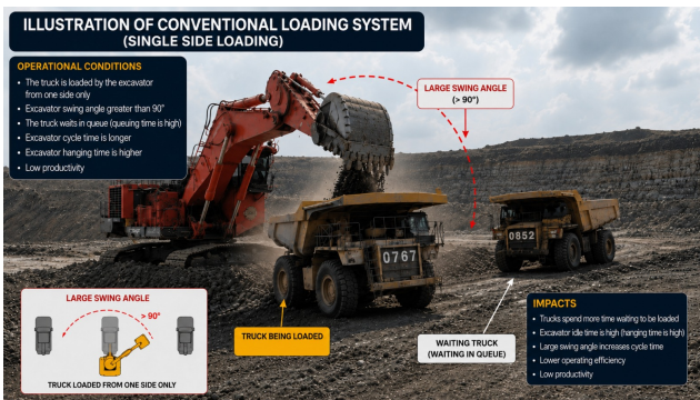
Figure 1. Existing single side loading configuration at the study site
